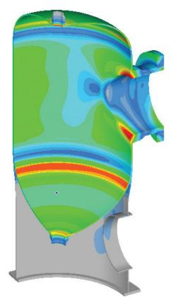
"Today, pressure equipment regulations allow us to apply a more accurate analysis method, using a tool like Femap with NX Nastran for nonlinear calculations."
