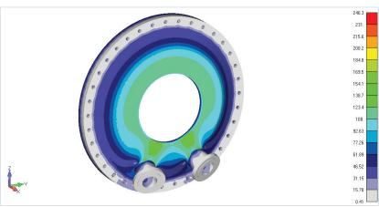
"The Femap nonlinear approach offers a wider admissibility range," Palloni adds. "With the same geometry and materials, a component can offer higher performance than those predicted with elastic linear analysis. Another benefit is obtained in the postprocessing phase, which is faster and immediate."
